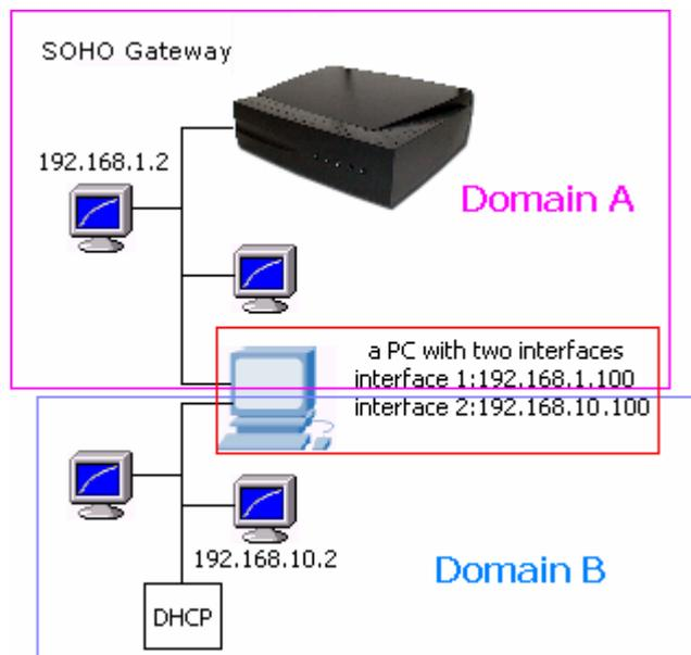
Figure 3-14 Static Routing
