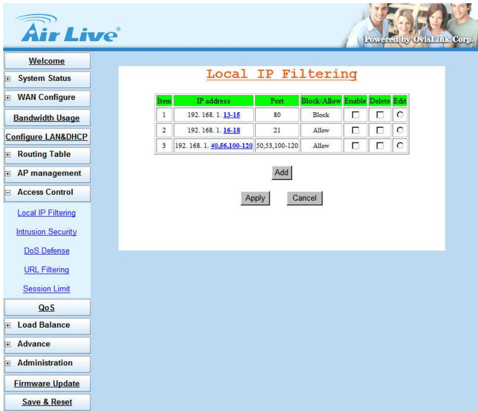
Figure 3-19 Local IP Filtering Example Setting
