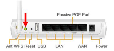
If you also have a hardware WPS button on your wireless card, you can push the button immediately now. If not, you can usually find the WPS PBC function in the wireless utility. Below is an example using AirLive WN-360USB wireless network card to connect with N.Power.
