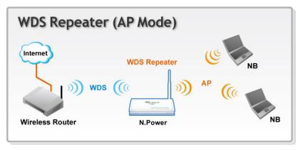
This is known as WDS Repeater function. In AP mode, the N.Power will repeat the wireless signal of remote AP/Router. Up to 4 WDS repeaters can be connect with N.Power. WDS works by entering the wireless MAC addresses (also known as BSSID) of remote Access Points.
