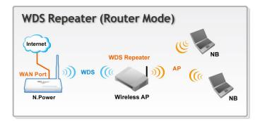
This is known as WDS Repeater function. Enable this setting to allow remote WDS equipped AP to extend the wireless signal of N.Power. Up to 4 WDS repeaters can be connect with N.Power. WDS works by entering the wireless MAC addresses (also known as BSSID) of remote Access Points.
