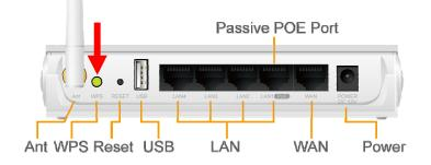
If you also have a hardware WPS button on your wireless card, you can push the button immediately now. If not, you can usually find the WPS PBC function in the wireless utility. Below is an example using AirLive WN-360USB wireless network card to connect with N.Power.
