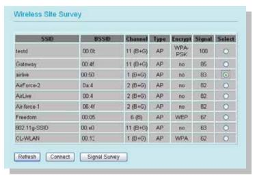
using the signal survey function. At last, the installer simply clicks on "connect" button to establish connection. The site survey is available even in AP mode, so the installer can check the channels used by surrounding APs to avoid interferences.
