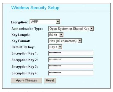
configure up to 4 keys using either ASCII or Hexadecimal format.
