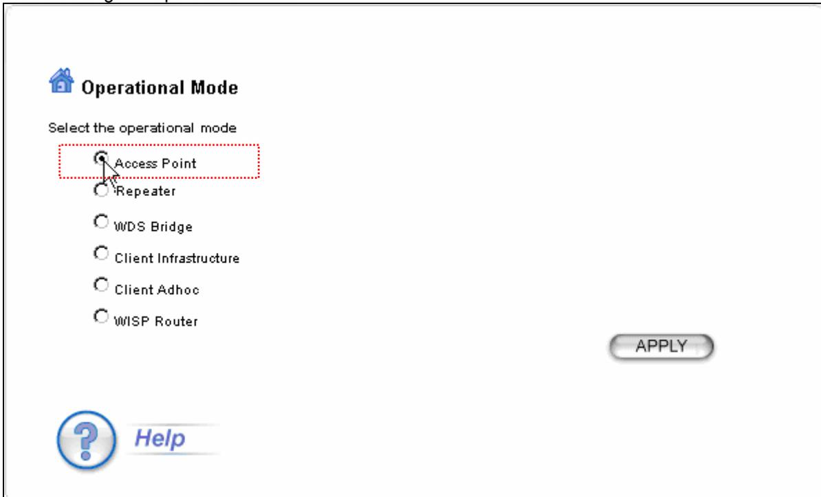
Set up first the device as an AP mode, click on “APPLY”,
