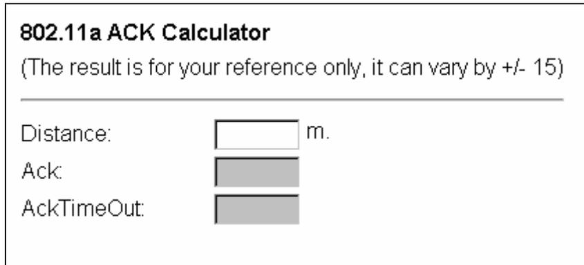
Input distance value in meters. The ACK Timeout value will be automatically calculated accordingly. This is the value to be entered into the "ACK Timeout (11a)" or "ACK Timeout (11g)" field according to the spectrum.
