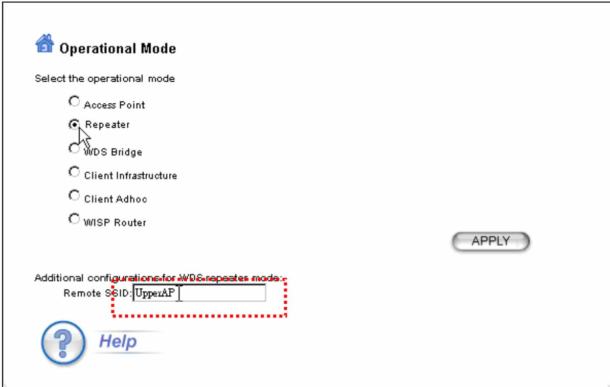
Select "Repeater" mode and then enter the "Remote SSID", this is the SSID of AP node's SSID.
