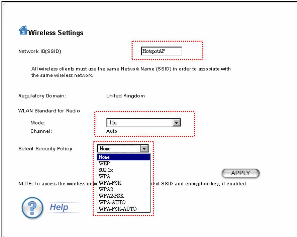
Set the SSID for the Hotspot service. This SSID can be different from upper node's SSID. Its Channel will be display as "Auto" it will be same as the AP node's channel. It's necessary to set the Wireless mode as the same spectrum as AP's node. You can set encryption for the security between hotspot services with client device.
