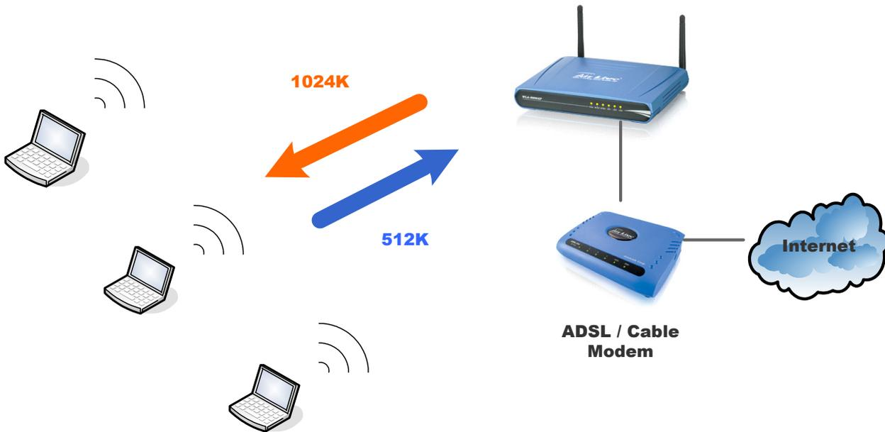
In this example, total uplink bandwidth of the 3 clients is limited to 512kbps and the total download bandwidth of the 3 clients is limited to 1024kbps.
