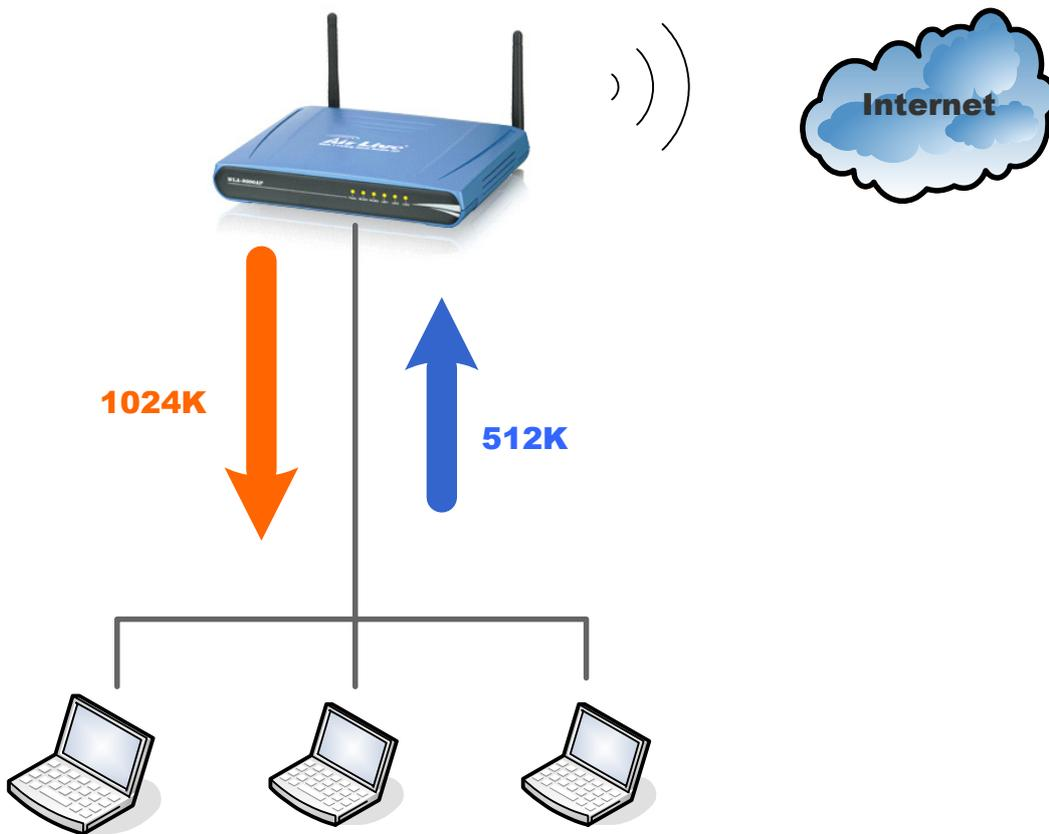
In this example, total uplink bandwidth of the 3 clients is limited to 512kbps and the total download bandwidth of the 3 clients is limited to 1024kbps.
