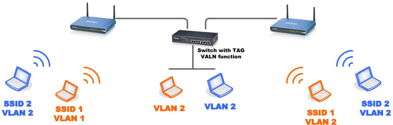
In the above example, laptops in VALN 1 can only communicate with those in VLAN 1 and laptops in VALN 2 can only communicate with those in VLAN 2.
