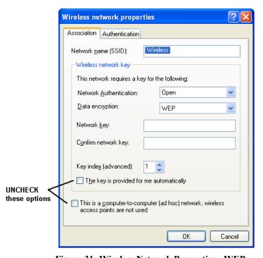
Figure 31: Wireless Network Properties - WEP
