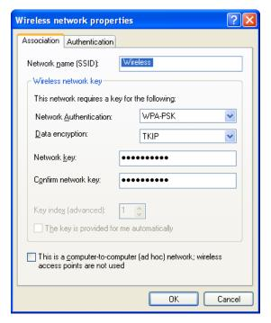
Figure 35: Wireless Network Properties- WPA-PSK
