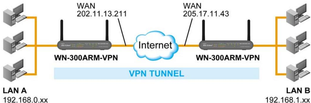
Figure: Connecting 2 WN-300ARM-VPN
