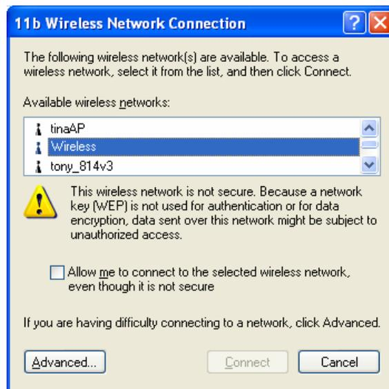
Figure: Insecure Wireless Network (Windows XP)
