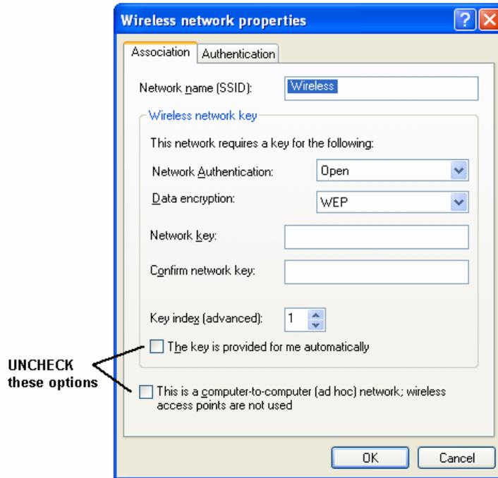
Figure: Wireless Network Properties - WEP
