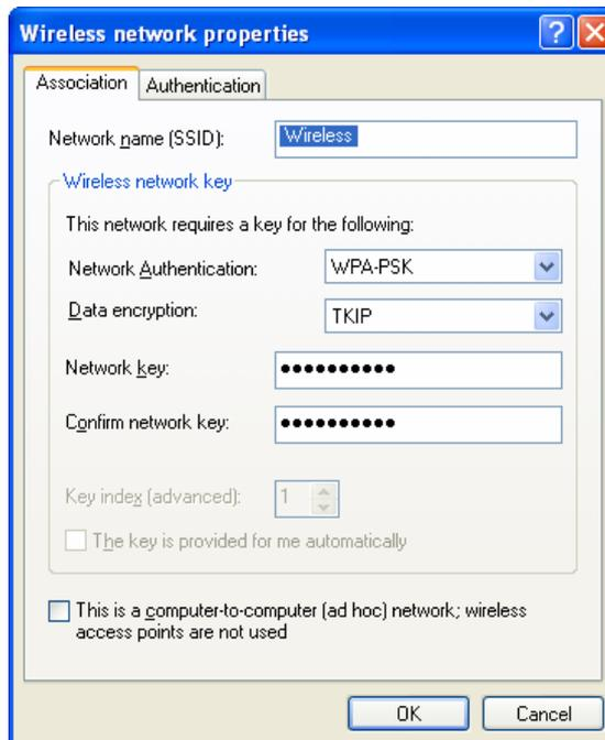
Figure: Wireless Network Properties- WPA-PSK
