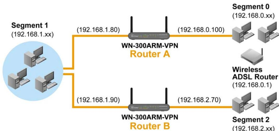
**Figure: Routing Example**
