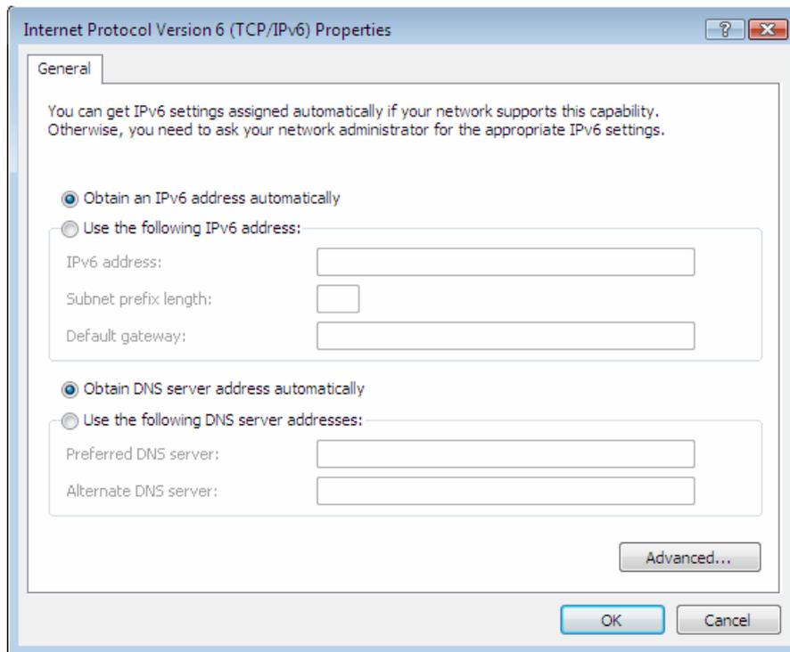
Figure: TCP/IP Properties (Windows Vista)
