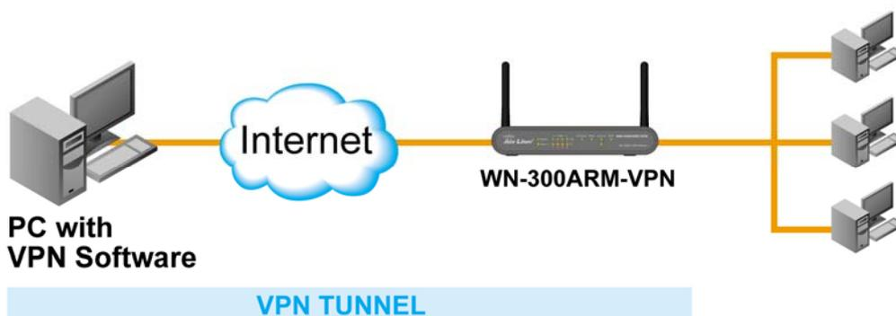
Figure: Client PC to VPN Gateway
