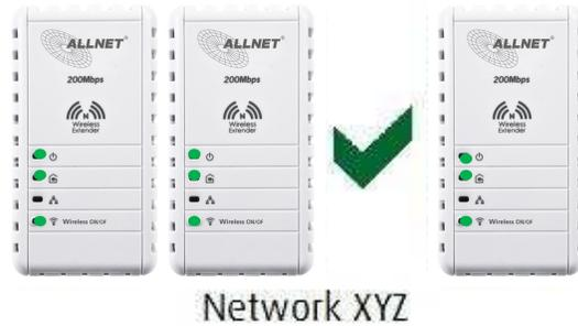
If the Powerline Activity LED
