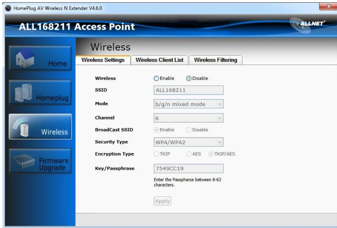
SSID: Displays the wireless SSID of the device.
