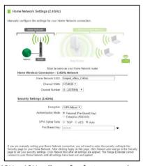
Channel Width: Wi-Fi operates in two separate channel widths, 20Hz and 40Hz. 40Hz allows for faster speeds. Each Channel Width will have a different selection of wireless channels to choose from. Select the channel width you wish to use for your network. This setting must match that of your Home Network for a successful connection.
