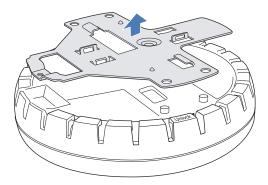
c. Turn over the universal mounting bracket, then align the bracket over the cable ports and the four mounting posts as shown in **Figure 2–29**.
