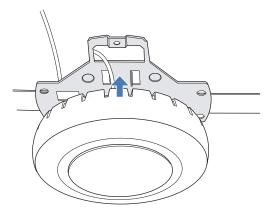
12. Lock the MP onto the bracket by inserting a small-pointed instrument or a paperclip into the **Lock** hole on the MP as shown in **Figure 2–9**.
