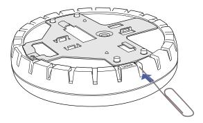
2. Remove the bracket as shown in **Figure 2–19**.
