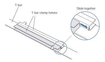
Figure 2-11. Step 3-Installing the T-bar Clamp for a 5/8-inch (15.9-mm) T-bar
