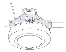
11. Lock the MP onto the bracket by inserting a small-pointed instrument or a paperclip into the **Lock** hole on the MP as shown in **Figure 2–17**.
