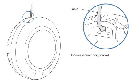
10. Lock the MP onto the bracket by inserting a small-pointed instrument or a paperclip into the **Lock** hole on the MP as shown in **Figure 2–26**.
