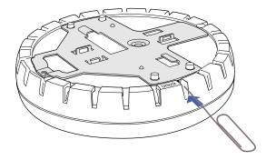
5. Remove the bracket as shown in **Figure 2–13**.
