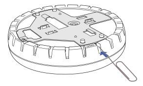
4. Remove the bracket as shown in **Figure 2–23**.
