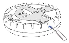
b. Remove the bracket as shown in Figure 2-28.
