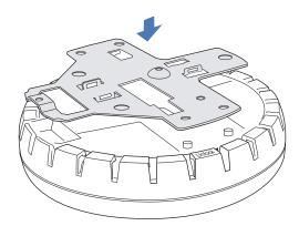
d. Once the bracket is fully seated, lock the bracket onto the MP by inserting a small-pointed instrument or a paperclip into the **Lock** hole on the MP as shown in **Figure 2–30**.
