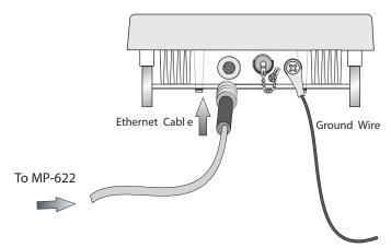
The MP-622 does not have a power switch. It is powered on when the Ethernet port is connected to the power injector module, and the power injector module is connected to an AC power source.
