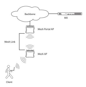
In the illustration, a client is associated with a *Mesh AP*, which is an MP without a wired interface to the network. The Mesh AP is configured to communicate with a *Mesh Portal AP*, an MP with wired connectivity to an MX. Communication between the Mesh AP and the Mesh Portal AP takes place over a secure radio link (a *Mesh Link*). When associated with the Mesh AP, the client has the same connectivity to the network as if the Mesh AP is using a wired link.
