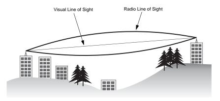
If there are obstacles in the radio path, there may still be a radio link but the quality and strength of the signal will be affected. Calculating the maximum clearance from objects on a path is important as it directly affects the decision on antenna placement and height. It is especially critical for long-distance links, where the radio signal could easily be lost.
