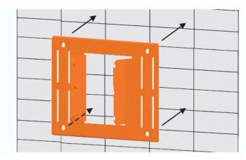
2. Position the bracket in the intended location and mark the position of the four mounting screw holes.
