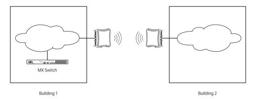
The wireless bridge is established between a Mesh Portal AP and a Mesh AP to which it is associated. The bridged data packets are those present on the Ethernet interfaces of the two MPs. A Mesh AP serving as a bridge endpoint picks up packets from a wired port and transfers them to the other bridge endpoint. A simple source/destination learning mechanism is used to avoid forwarding packets across the bridge unnecessarily.
