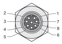
Table 5-2. 8-Pin DIN Ethernet Port Pinout
