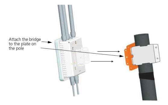
5. Use the included nuts to secure the wireless bridge to the pole bracket. Note that the wireless bridge tilt angle may need to be adjusted during the antenna alignment process. Be sure to take account of the antenna polarization direction. All antennas in a link must be mounted with the same polarization.
