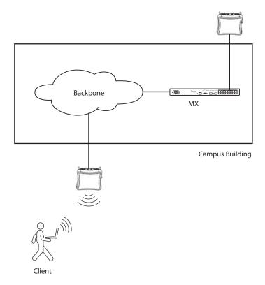
The MP-622 can be connected directly to an MX or indirectly over the network.
