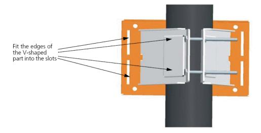
3. Attach the adjustable rectangular plate to the bridge with supplied screws.
