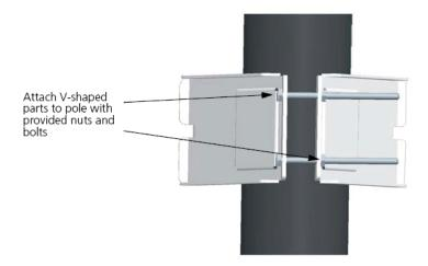
2. Fit the edges of the V-shaped part into the slots in the rectangular plate, and use the included nuts to tightly secure the MP-622 to the bracket.
