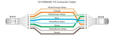
EIA/TIA 568B RJ-45 Wiring Standard
