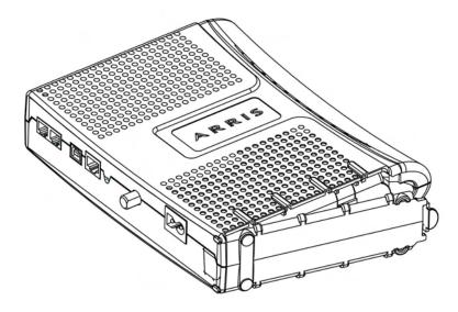
Replace the door. To do so, place the tabs of the battery door into the slot on the Telephony Modem battery compartment. Rotate the door toward the front of the Telephony Modem until the latch snaps back into place.
