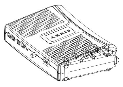
4 Replace the door. To do so, place the hinge tabs of the battery door into the receiver slots inside the Telephony Modem battery compartment on the opposite end of the battery opening slot. Rotate the door toward the unit until the latch snaps back into place.
