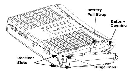
3 Push the battery pack into the bay until it latches into place. The following diagram shows a Telephony Modem with a 4.4 Ah lithium - Ion battery pack installed. If you are taking the battery out of the Telephony Modem, use the battery pull strap to dislodge the battery.
