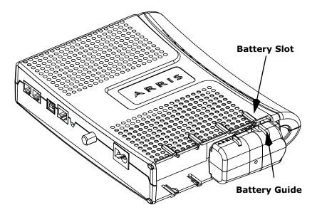
2 Hold the battery pack so that the guides on the battery align with the slots on the Telephony Modem and slide the battery into the bay. The diagram on the left shows the proper orientation.
