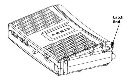
2 Hold the battery pack so that the guides on the battery align with the slots on the Telephony Modem and slide the battery into the bay. The diagram on the left shows the proper orientation.
