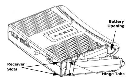
3 Push the battery pack into the bay until it seats into place. The following diagram shows a Telephony Modem with a 2.2Ah battery pack installed. If you are taking the battery out of the unit, position your finger in the battery opening area and use leverage to dislodge the battery while pulling it straight back.
