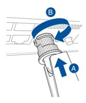
2. Align the projecting point on the bush to the notch on the sliding sleeve, and push the bush into place.
