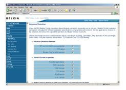
Network attacks that deny access to a network device are called DoS attacks. DoS attacks are aimed at devices and networks with a connection to the Internet. Their goal is not to steal information, but to disable a device or network so users no longer have access to network resources.
