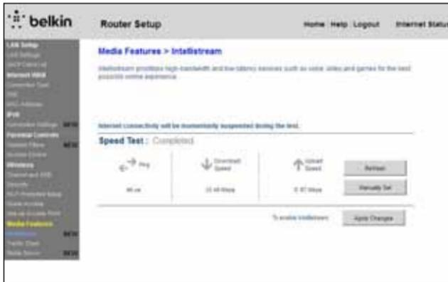
The screenshot shows the Belkin Router Setup interface. The left sidebar contains navigation options: LAN Setup, WAN, Firewall, Advanced, and Media Features. The main content area is titled "Media Features > IntelliStream". It includes a warning about internet connectivity suspension during the test and a "Speed Test: Completed" section. The test results are displayed as follows:
