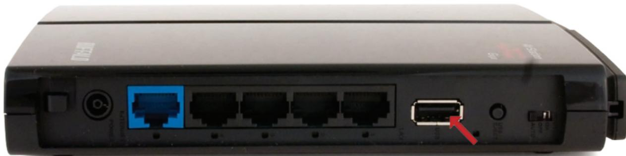
To add a USB hard drive or flash drive to the AirStation, plug it in to the AirStation's USB port.
