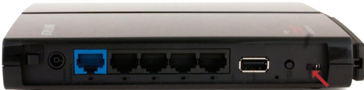
The AirStation may be used as either a full wireless router or a simple access point. The switch has three positions:
