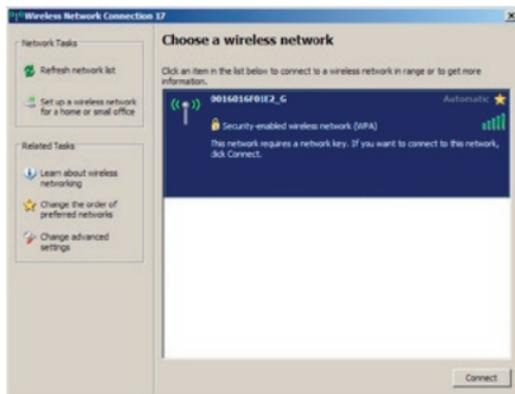
Any wireless networks available in the area will be listed as available. Click on your wireless network SSID so that it turns blue and then click on *Connect* at the bottom right.
