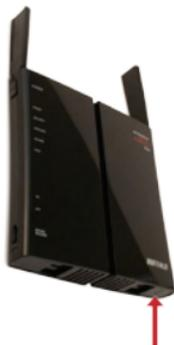
You may also initialize your AirStation by holding down the *Reset* button on the bottom for 3 seconds with a straightened-out paper-clip or similar object.
