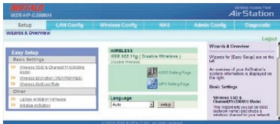
The Setup page is the opening screen of the Web Configuration Tool. From here, you can change your wireless SSID and channel, and choose your encryption type under Basic Settings. The *Wireless Config* section also shows your SSID and encryption settings.
