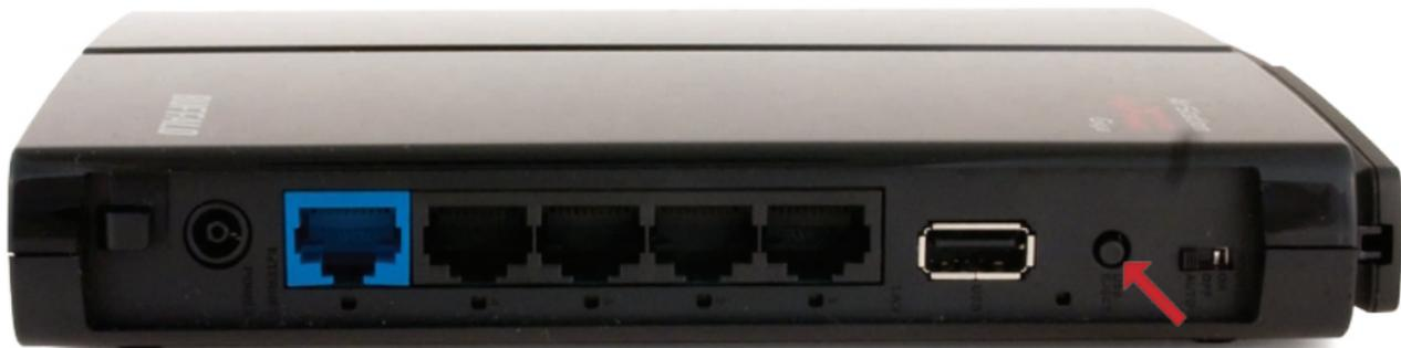
To release the USB device, hold down the USB Release button for 3 seconds. The USB device will be dismounted. When the USB LED stops blinking, it is safe to unplug the USB drive.
