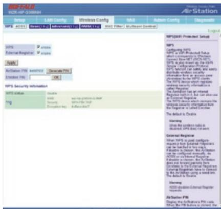
**Method # 2:** If your wireless client requests a PIN code, enter the AirStation's PIN code. You can get it from the sticker on the back of the AirStation, or from the WPS page in the Web Configuration tool.
