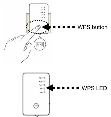
(2) Press the **WPS button** on the wireless broadband router or access point you wish to connect to within 2 minutes.
