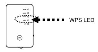
(2) Press the **WPS button** on the wireless client you wish to connect to within 2 minutes.
