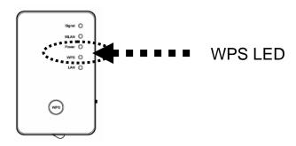
When quick installation is successful, the 'Signal' LED will turn on.
