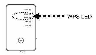
When quick installation is successful, the 'Signal' LED will turn on.
