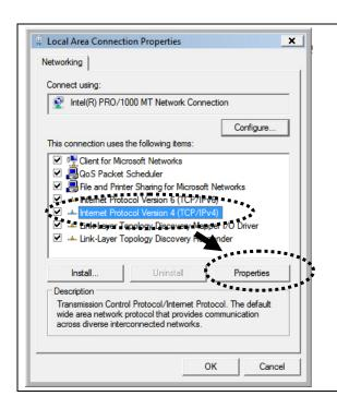
Click the 'Start' button (it should be located at the lower-left corner of your computer screen), then click the control panel. Click *View Network Status and Tasks*, then click *Manage Network*Connections. Right-click *Local Area Network*, then select 'Properties'. The Local Area Connection Properties window will appear, select 'Internet Protocol Version 4 (TCP / IPv4), and then click 'Properties'
