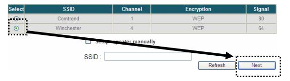
(5) If the Wireless Router or Access Point you're connecting to is using encryption, you'll be prompted to input the access point's wireless security key. Input it in the 'KEY' field and click the 'Next' button to continue.
