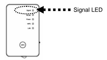
(4) Please move the Wireless-N Range Extender to the place you wish to use it (the ideal place will be the center of your house) and plug this Wireless-N Range Extender into a power outlet on the wall, the wireless connection will be established automatically as long as it's within range of your wireless router or access point.
