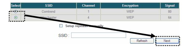
(5) If the Wireless Router or Access Point you're connecting to is using encryption, you'll be prompted to input the access point's wireless security key, input it in the 'KEY' field and click the 'Next' button to continue.
