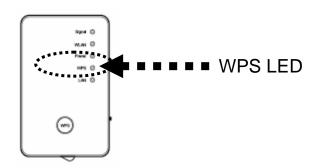
(2) Press the **WPS button** on the wireless broadband router or access point you wish to connect to within 2 minutes.
