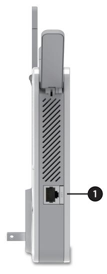
1 LAN Port Attach an Ethernet cable to either extend an existing wired network or convert a wireless network into a wired network.
