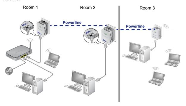
Figure 3. Powerline access point connected to the Powerline network and wireless network
