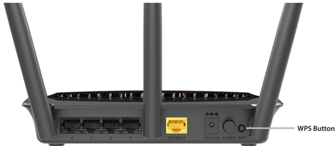
**Step 2** - Within two minutes, press the WPS button on your wireless client (or launch the software utility and start the WPS process).
