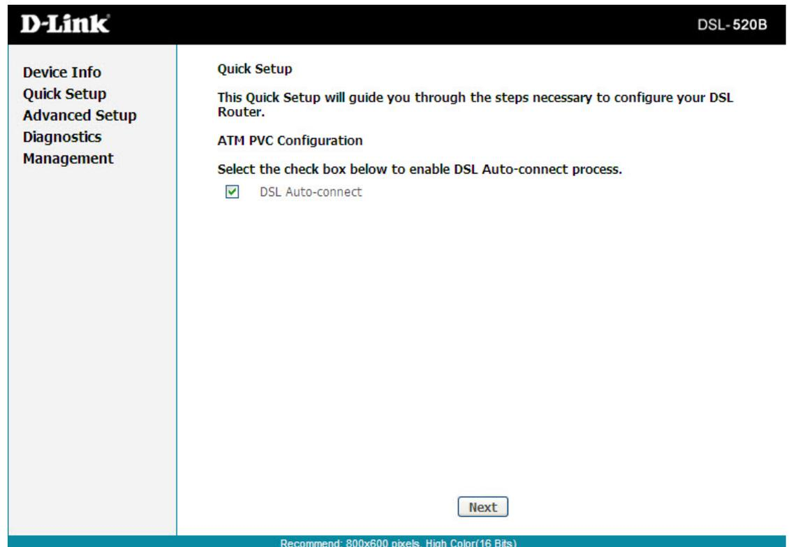
The router will automatically perform a PVC scan in order to detect your DSL connection.
