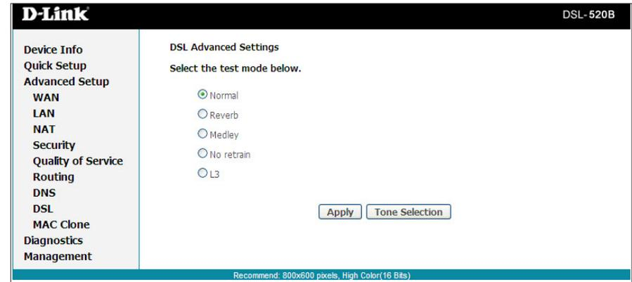
The frequency band of ADSL is split into 256 separate tones, each spaced 4.3125 kHz apart. Each tone carries separate data, so the modem operates as if 256 separate modems were running in parallel. The tone range is from 0 to 31 for upstream and from 32 to 255 for downstream. Do not change these settings unless directed by your ISP.
