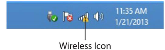
Clicking on this icon will display a list of wireless networks which are within connecting proximity of your computer. Select the desired network by clicking on the network name.
