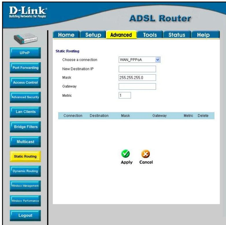
The screenshot shows the D-Link ADSL Router web interface. The top navigation bar includes 'Home', 'Setup', 'Advanced' (highlighted), 'Tools', 'Status', and 'Help'. A left sidebar contains various configuration options, with 'Static Routing' highlighted in yellow. The main content area is titled 'Static Routing' and contains the following fields:
