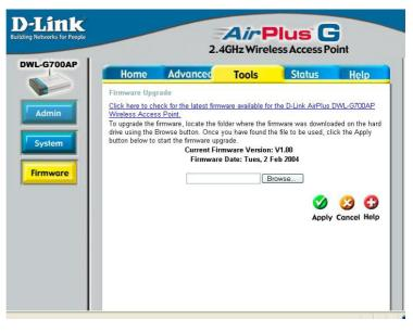
This screen displays the current firmware version, and the current wireless and Ethernet settings of the DWL-G700AP.
