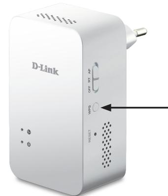
**Step 2** - Within 2 minutes, press the WPS button on your wireless client (or launch the software utility and start the WPS process).
