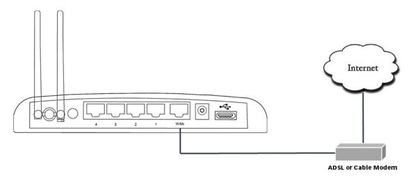
Connect all your computers, network devices (switch / hub) to the LAN port of the router.
