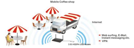
After connecting into the router, 3G USB Modem will be regarded as the fifth WAN port. However, the other Ethernet WAN ports still can be used and Load-Balance can be done in the router. Besides, 3G USB Modem also can be used as backup device. Therefore, when other Ethernet WAN ports are not available, the router will use 3.5G for supporting automatically. The supported 3G USB Modem will be listed on DrayTek web site. Please visit www.DrayTek.com for more detailed information.
