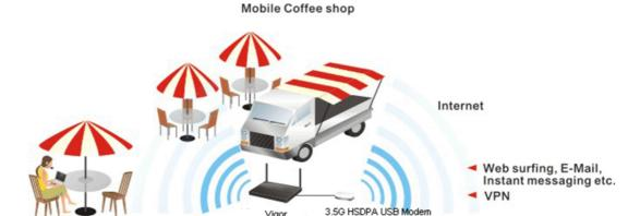
After connecting into the router, 3G USB Modem will be regarded as the fifth WAN port. However, the other Ethernet WAN ports still can be used and Load-Balance can be done in the router. Besides, 3G USB Modem in WAN5 also can be used as backup device. Therefore, when other Ethernet WAN port is not available, the router will use 3.5G for supporting
