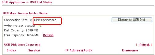
Note: If the write protect switch of USB disk is turned on, the USB disk is in READ-ONLY mode. No data can be written to it.
