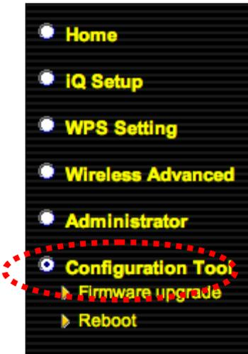
The wireless bridge’s configuration tool enables you to back up or restore the settings, upgrade the firmware and reset the device. Select “Configuration tool” from the sidebar.
