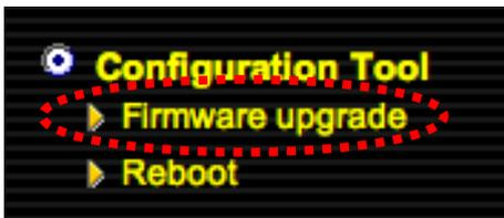
Selecting “Firmware upgrade” from the “Configuration Tool” menu allows you to update the system firmware to a more recent version. You can download the latest firmware from the Edimax website.
