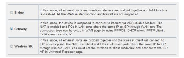
The **Gateway** mode allows that the first Ethernet port is treated as WAN port and the Ethernet port and the wireless interface are bridged together and are treated as LAN ports.
