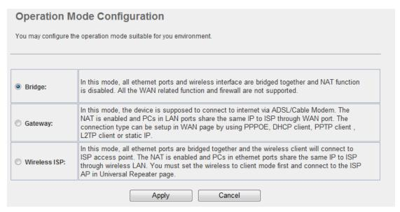
The **Bridge** mode allows that all Ethernet and wireless interfaces are bridged into a single bridge interface.
