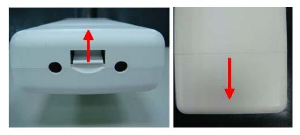
Step2: Pass through Ethernet cable from the hole, insert the cable to Secondary port.
