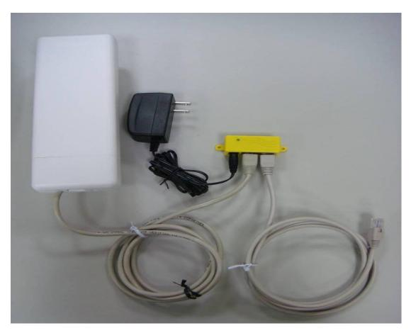
Notes: Use **Reset button** on POE injector. Push continually the reset button of POE injector about 5 ~ 10 seconds to reset the configuration parameters to factory defaults.
