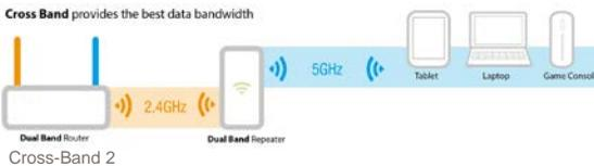
5GHz WiFi clients connected to the EM4596 and the EM4596 connected to the modem/router by 2.4GHz (see picture Cross-Band 2)
