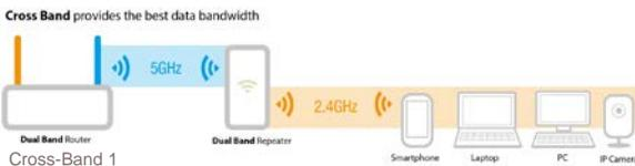
2.4GHz Wi-Fi clients connected to the EM4597 and the EM4597 connected to the modem/router by 5GHz (see picture Cross-Band 1)
