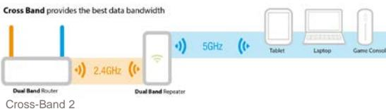
5GHz Wi-Fi clients connected to the EM4597 and the EM4597 connected to the modem/router by 2.4GHz (see picture Cross-Band 2)
