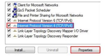
Select Use the following IP address and enter an IP address that is different from the EAP600 and subnet mask then click OK.
