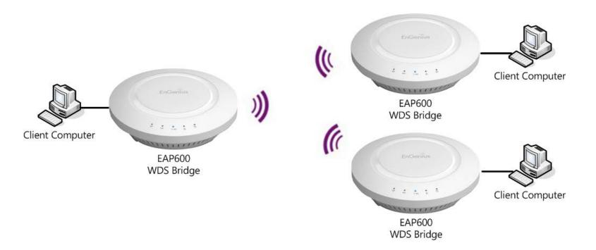
**Note**: WDS Bridge Mode does not act as an Access Point. Access Points linked by WDS are using the same frequency channel. More Access Points connected together may lower throughput. This configuration can be susceptible to generate endless network loops in your network, so it is recommended to enable the Spanning Tree function to prevent this from happening.
