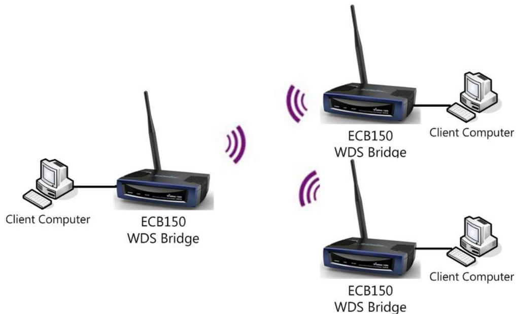
**Note:** WDS Bridge Mode does not act as an Access Point. Access Points linked by WDS are using the same frequency channel. More Access Points connected together may lower throughput. Please be aware to avoid loops in your wireless connection, otherwise enable Spanning Tree Function.
