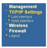
Click on the TCP/IP Settings link on the navigation drop-down menu. You will then see two options. Usijng this menu you may configure the LAN IP address, DHCP, Static or Dynamic WAN IP and PPPoE. Each option is described below.
