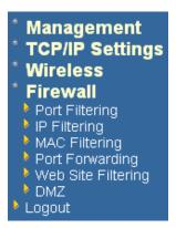
Click on the Firewall link on the navigation drop-down menu. You will then see six options. Port filtering, IP filtering, MAC filtering, Port filtering, URL filtering, DMZ. Each option is described below.
