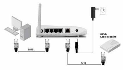
Figure 4: Wired Connection Diagram
