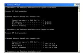
The default gateway represents the IP address of your GN-BR02G, that is: 192.168.1.254. All computers accessing this Router MUST be in the same subnet (192.168.1.x, where x is anything between 1 and 253) In the above example, the BR02G gateway shown above is 192.168.1.254, and the PC's IP address is 192.168.1.2
