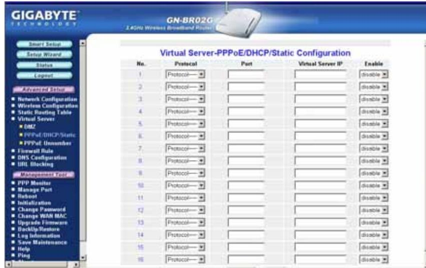
The BR02G is configurable to behave as a Virtual Server, allowing remote computers on the WAN (Internet) side of the network to be automatically redirected to local server(s) on the LAN (your private network) side of the network.
