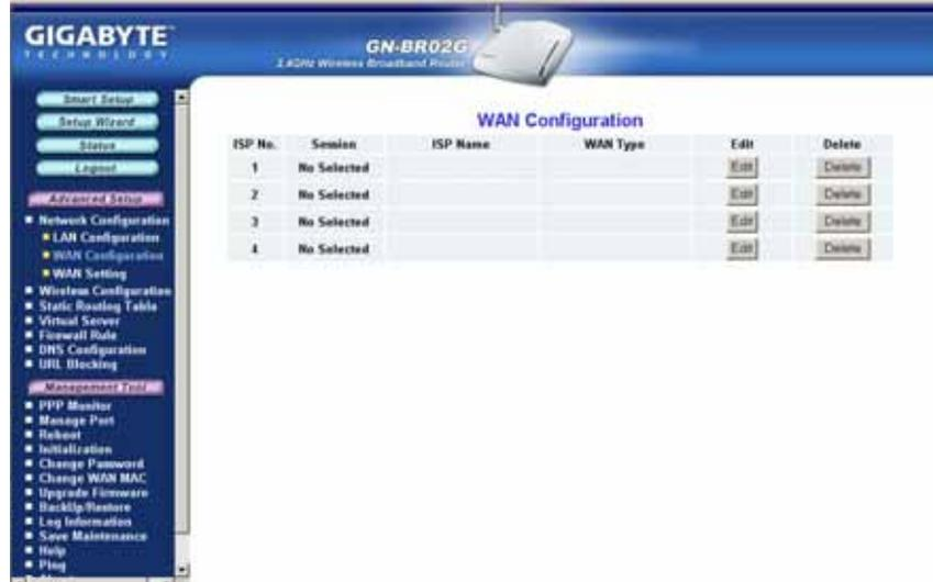
The BR02G has many advanced WAN configuration features. As a special redundant feature, you can configure up to 4 WAN connections and each may have its own connection type (PPPoE, PPPoE Unnumber, Dynamic IP address, Static IP address) and other properties. The device can automatically attempt to connect to these in order if your primary connection fails.
