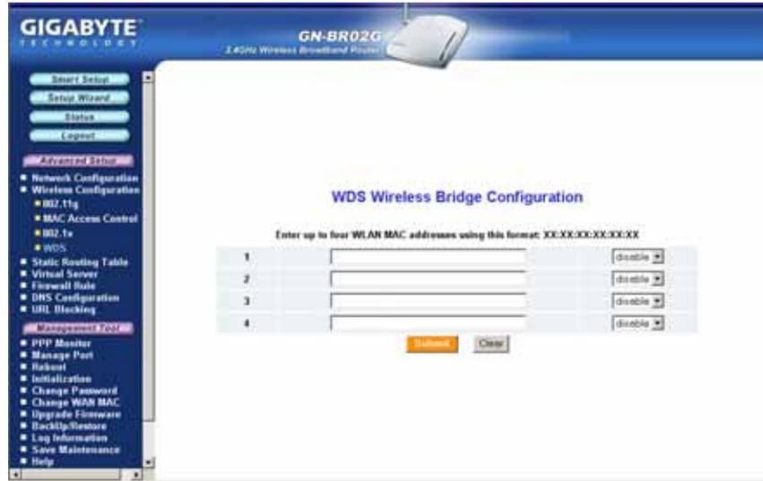
Wireless Distribution System (WDS) technology enables several access points to increase the coverage of a wireless network. Although enterprises or home users can reduce most wiring problems by using access points that support WDS, they still need cables to connect external ISP.
