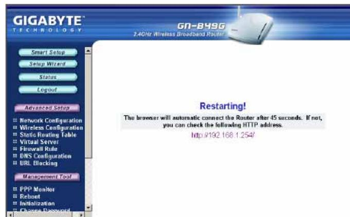
Once your router has successfully rebooted, it will load Router Welcome Screen. **Setup is complete.**
