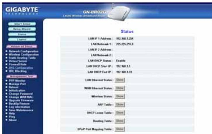
**LAN IP 1 Address** Displays the primary IP address being used by the Local (LAN) port of the Router. The default is 192.168.1.254
