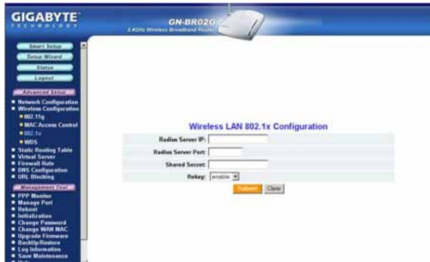
Your BR02G supports 802.1x and RADIUS Server authentication. RADIUS provides a centralized, server-based authentication of client access to the network.
