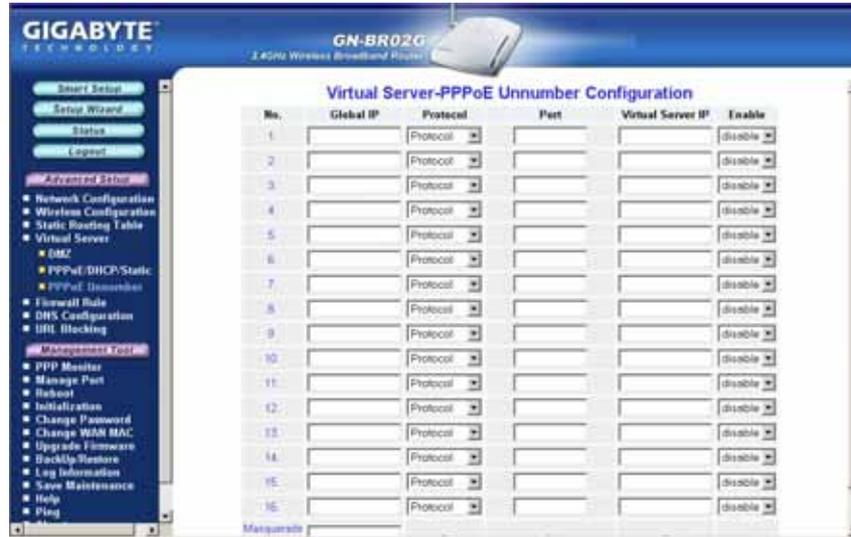
Advanced feature of the BR02G is that it supports services that offer multiple global IP addresses, with each IP address requires its own setting. This feature is normally only found on enterprise class routers. The BR02G has an IP allocation scheme capable of directly assigning global IP to LAN clients.
