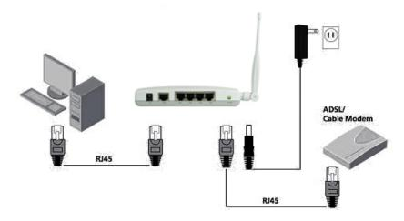
Figure 5: Wired Connection Diagram
