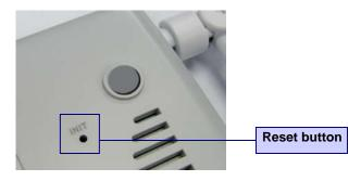
Figure 2: Router's Bottom Panel
