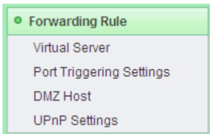
The submenus of the **Forwarding Rule** include **Virtual Server**, **Port Triggering Settings**, **DMZ Host**, and **UPnP Settings**.
