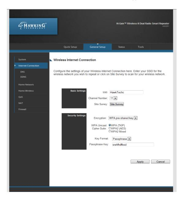
You may manually enter the SSID of the wireless network you plan on connecting to or you can click 'Site Survey' to have the web interface scan for local networks in your vicinity. (See Site Survey Menu below)
