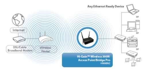
AP Bridge – Point to Point: Similar to station-infrastructure, this requires two HWABN2's on each end. This will create a wireless bridge between these two points. No WiFi signal will be broadcast and it will only make a wireless connection between those two points.
