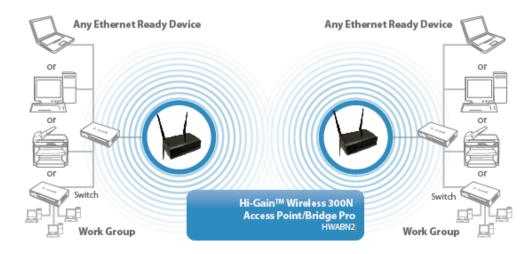
**AP Bridge – Point to Multi-Point:** Similar to AP Bridge – Point to Point, this allows you to connect several HWABN2's to one point. No WiFi signal will be broadcast and it will only make a wireless connection between the HWABN2s.
