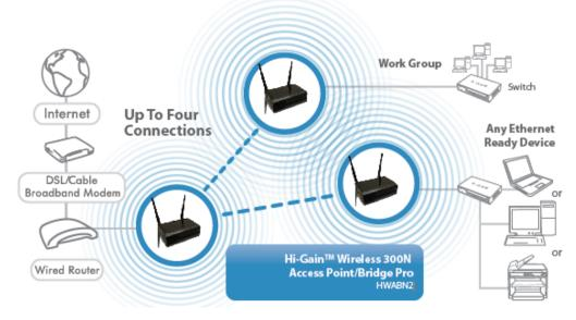
**AP Bridge WDS**: Wireless Distributing System. This allows you to create a wireless network using up to four HWABN2's using the same SSID (wireless name). It will broadcast a WiFI signal.
