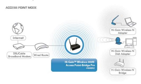
**Station – Infrastructure (Bridge):** The HWABN2 will allow you connect wired devices wirelessly to an existing wireless router or access point. It will "bridge" these devices wirelessly with your network. It will not broadcast any WiFi signal. It will only make a wireless connection between the Access Point and the HWABN2.
