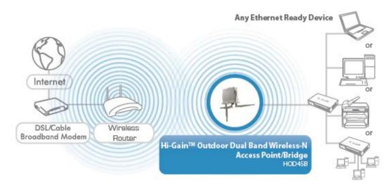
**AP Bridge** – **Point to Point:** Similar to station-infrastructure, this requires two HWABN25's on each end. This will create a wireless bridge between these two points. No WiFi signal will be broadcast and it will only make a wireless connection between those two points.
