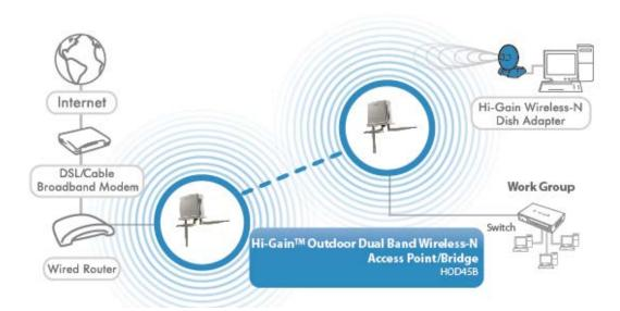
**Universal Repeater:** In this mode, the HWABN25 will repeat the wireless signal of any existing wireless router/access point. It will act as a wireless relay and create a larger
