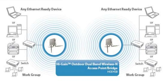
**AP Bridge** – **Point to Multi-Point:** Similar to AP Bridge – Point to Point, this allows you to connect several HWABN25's to one point. No WiFi signal will be broadcast and it will only make a wireless connection between the HWABN25s.
