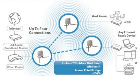
**AP Bridge WDS**: Wireless Distributing System. This allows you to create a wireless network using up to four HWABN25's using the same SSID (wireless name). It will broadcast a WiFI signal.
