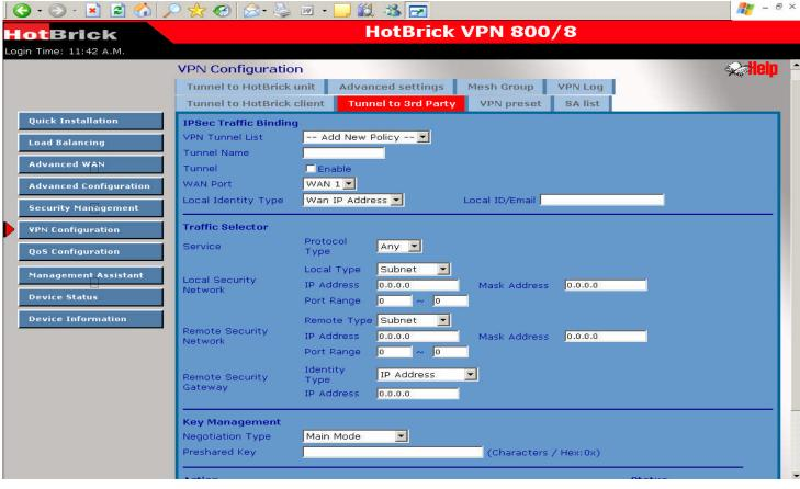
Tunnel to 3rd Party - This describes an IPsec tunnel from a VPN800/8 F with a non-Hotbrick certified unit.
