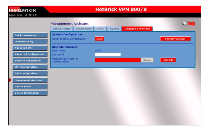
This Upgrade Firmware Screen allows you to upgrade firmware on the system, to enable remote administration, and FTP upgrade.
