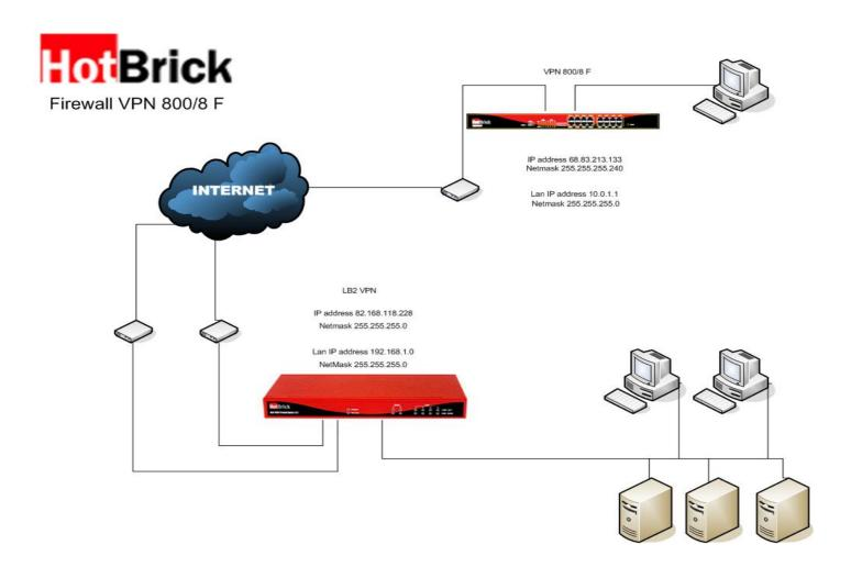
This example takes a tunnel between a VPN 800/8 F and a LB-2 VPN. This example applies to the HotBrick 401VPN X2, LB-2 VPN and 800/8 F series, you can use either unit at both sides. You can use the IP addresses from the network diagram above.
