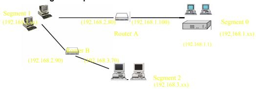
The VPN 800/8 F Firewall Gateway's Routing Table
