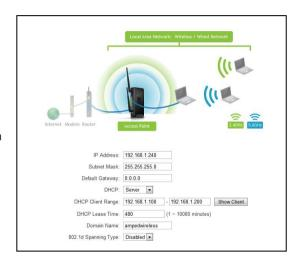
Note: If you choose to use a Static IP address for the Access Point, you will no longer be able to access the web menu using http://setup.ampedwireless.com. You must use the assigned IP address to acces the web menu.
