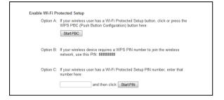
Option A: Push button: You may push the WPS button on the web menu or use the physical button on the back of the Access Point.
