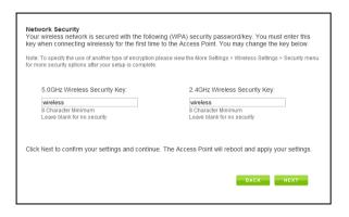
Click Next to complete the setup process. The Access Point will reboot and apply your settings. Be patient and do not make any changes or adjustments to the Access Point at this time.
