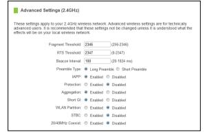
Beacon Interval: Indicates the frequency interval of the beacon. A beacon is a packet broadcast by the router to synch the wireless network.
