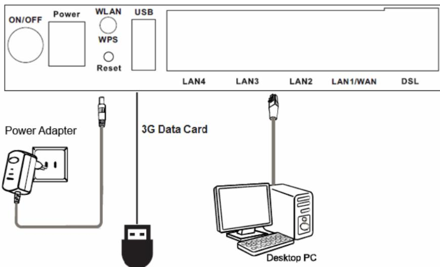
**Note:** SIM card is properly inserted & ISP Service is activated before inserting USB modem into the router
