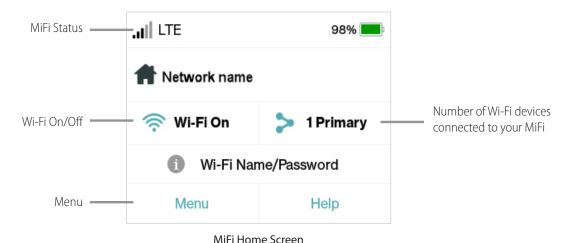
At the top of the screen, you'll see status indicators for network signal strength **...!!**, data traffic activity **...**, unread system messages **...**, roaming **...**, and battery **...**.
