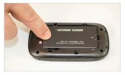
Replace the cover by setting it on the MiFi 7000 where the notches align, then press on the cover until it clicks into place and is flat across the entire bottom surface.
