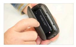
2 Insert your finger into the battery removal divot and lift the battery out of the battery compartment.
