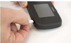
**CAUTION!** Do not bend or scratch your SIM card. Avoid exposing your SIM card to static electricity, water, or dirt.
