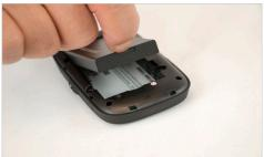
**3** Align the gold contacts on the new battery with the gold contacts on the MiFi 7000 and gently slide the battery into place.
