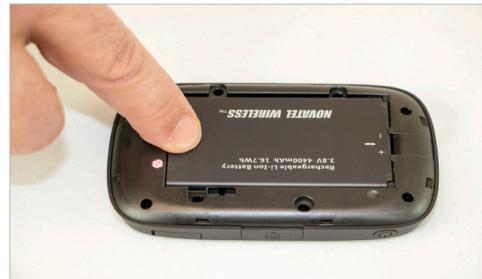
Replace the cover by setting it on the MiFi 7000 where the notches align, then press on the cover until it clicks into place and is flat across the entire bottom surface.
