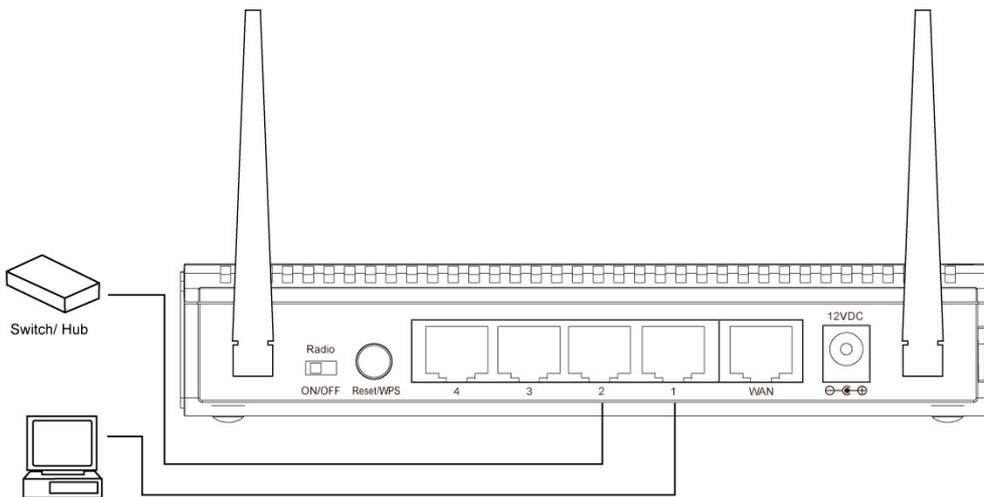
4. Connect the AC power adapter to the wall socket, then connect it to the Power socket of the router.
