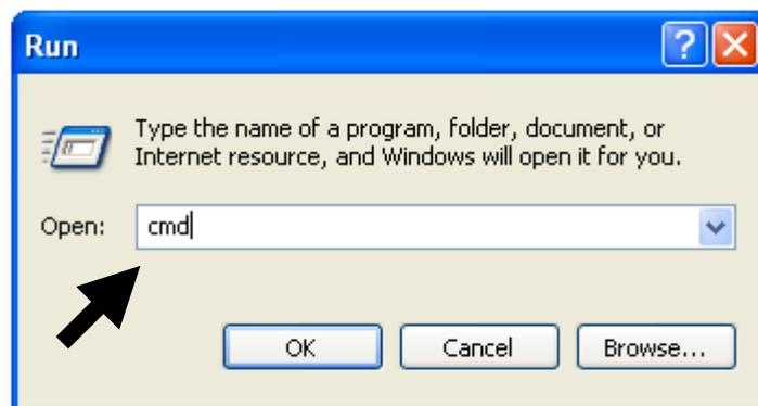
Input “ipconfig,” then press <Enter>. Check the IP address followed by the default gateway (in this example, the IP address of the router is 192.168.2.1).
