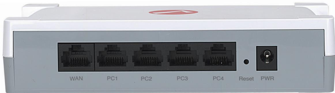
**WAN** — This 10/100Mbps port connects the cable/DSL modem.
