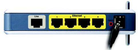
**Figure 4-3: Connect the Power**
