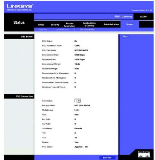
Figure 5-46: DSL Connection
