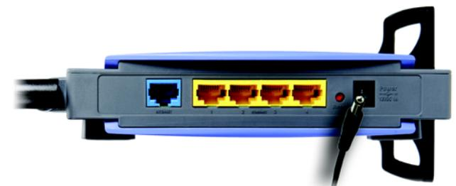
**Figure 4-3: Connect the Power**
