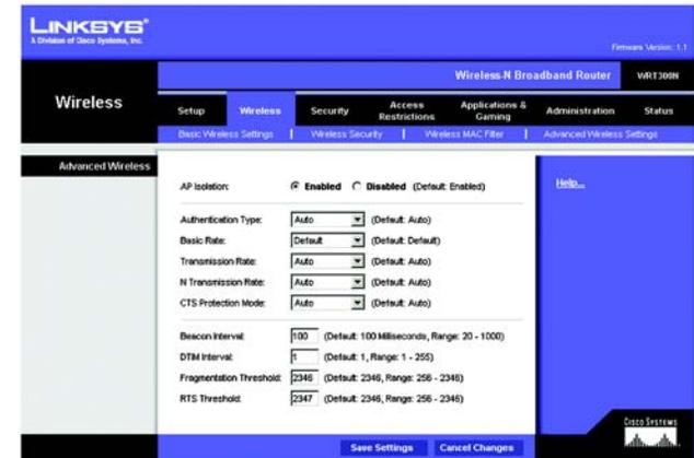
Figure 5-23: Wireless Tab - Advanced Wireless Settings
