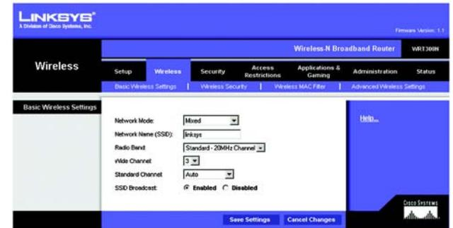
Figure 5-14: Wireless Tab - Basic Wireless Settings
