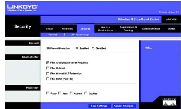
Figure 5-24: Security Tab - Firewall
