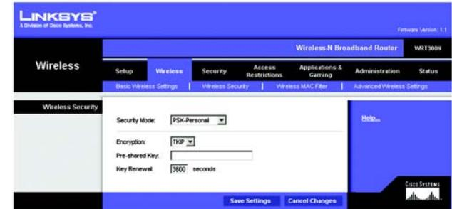
Figure 5-15: Wireless Tab - Wireless Security (PSK-Personal)
