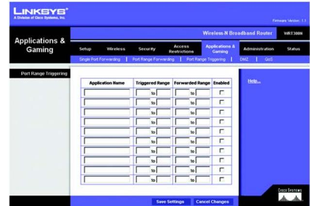
Figure 5-31: Applications & Gaming Tab - Port Range Triggering
