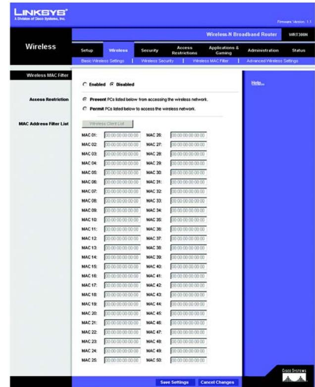
Figure 5-21: Wireless Tab - Wireless MAC Filter
