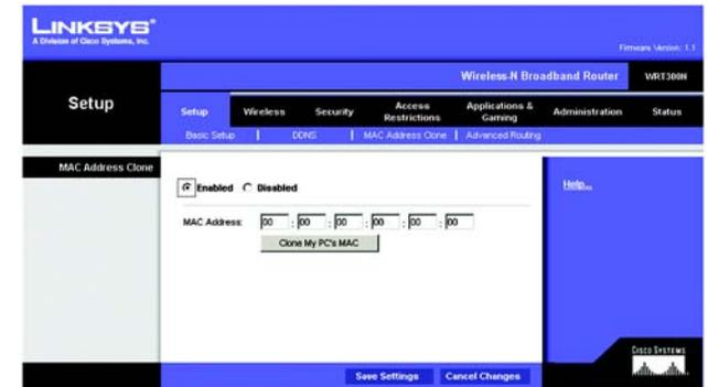
Figure 5-11: Setup Tab - MAC Clone
