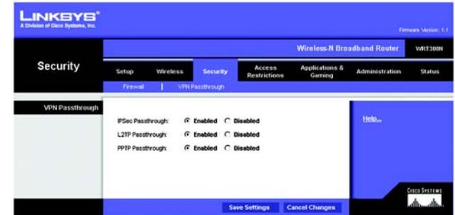
Figure 5-25: VPN Passthrough
